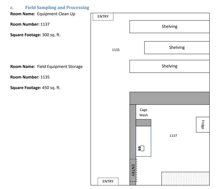
**Descriptions/Needs:** This area is used for initial field sample arrival and temporary storage. The room features clean and dirty areas to provide an area for initial sample arrival and sorting and a clean area for equipment and supply storage. There is a large floor sink suitable for washing coolers, traps, etc. Refrigerators and freezers are available for overnight sample storage.
